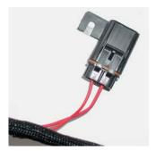
This fuse protects the ECU electronics. Back\_to\_Vehicle\_Battery\_Fuse
