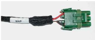
used. For blown or turbocharged applications a 2 BAR MAP sensor must be used for boost pressures up to 15 PSI. For boost pressures up to 30 PSI a 3 BAR MAP sensor must be used. If a 2 or 3 BAR MAP sensors are used, the harness side MAP sensor connector can be easily modified (or replaced). The modification involves cutting a new key-way in the connector Contact a BigStuff
