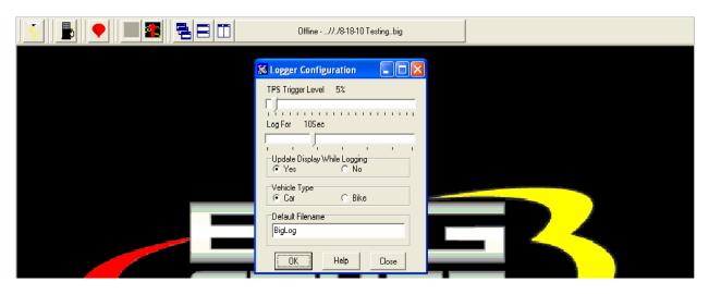
Using the Throttle Position Sensor (TPS) as a Load input, the user can automatically trigger the BigComm software's data-logging feature. Place the left mouse cursor on the "TPS Trigger Level" slide bar. Depress the left mouse button and slide it to the desired TPS % value or threshold. The logging feature will automatically start once the selected % TPS value is exceeded.
