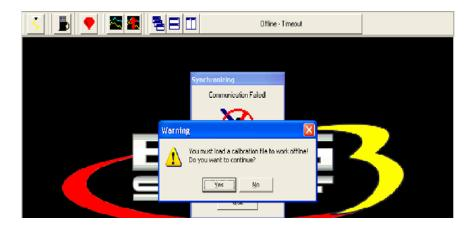
Left mouse click on Yes and the BigComm software should go to the BigComm folder. If the PC does not automatically take you to the BigComm folder, navigate to **C: Program**
