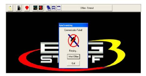
If the GEN3 ECU is not powered up (the ignition key is not in the "Run" position) and the Communications cable is not connected, communication cannot be established. The following screen will appear. This may also occur if the Comm Port is not configured correctly. If this occurs, use the above process of configuring the Comm Port until communication is established.
