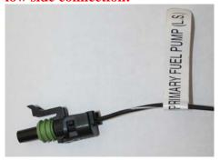
This connector <u>must</u> go to the negative side of a fuel pump relay, not directly to the fuel pump.
