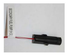
This connector <u>must</u> go to the positive side of a fuel pump relay, not directly to the fuel pump.
