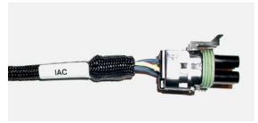
connector is the factory installed IAC, the 2-by-2-connector can be removed and replaced with a 4-by-1 inline connector per the pin-out table below. The 1-by-4 connector is available from BigStuff3. The LS1/LS7/Ford Mod Motor systems main harness IAC connector is a 1x4 GM style IAC motor connector.
