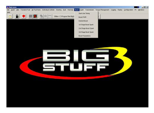
Keep the left mouse button depressed and slide the mouse pointer down until "Boost Parameters" is highlighted. Release the left mouse button. The screen below will open.
