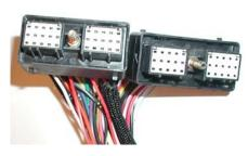
To avoid the potential of severely damaging the ECU, connect the head connectors to the ECU only after the battery connections are made. The two 30-way MWH header connectors are keyed such that they will only fit in only one (1) of the two (2) ECU mating-half connectors. To fasten the MWH connectors to the ECU, use a 1/4-nut driver. Make sure the header connectors, on all the harnesses, are tightened to 15 - 20 in lbs. Do not over-tighten
